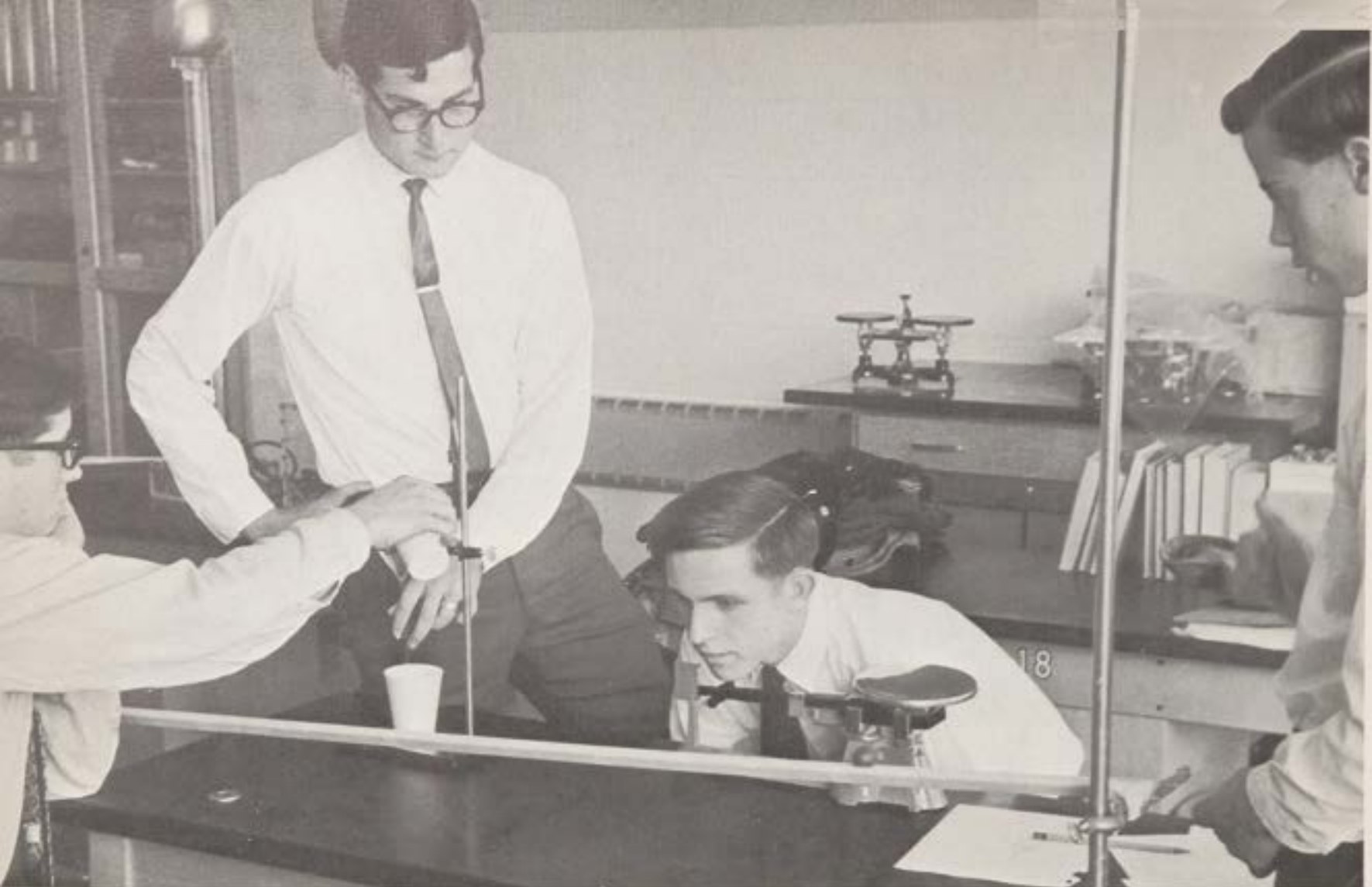
Using a water clock and Galileo's analysis of acceleration, R. Tort measures the time for a ball to roll down an incline in Cultural Physics Lab.
