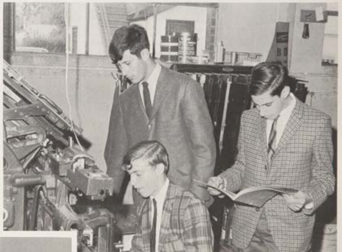
Typists E. Masson, H. Caplan, and T. Florczak are interested in the Linotype machine, which transfers letters into print.
