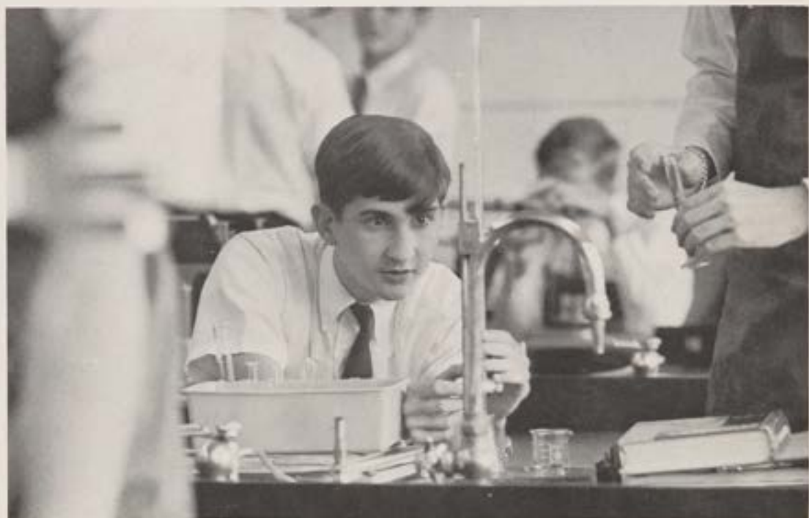
K. Kuker utilizes a burette to discover the molarity of an unknown acid solution.
